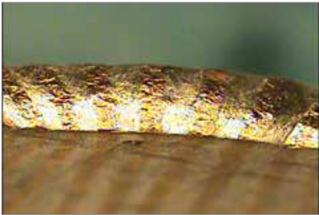
Figure 9 14K Red/Sterling billet: no de-lamination
