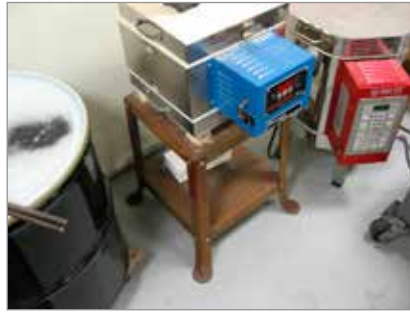
Figure 2 Ovens used for firing and annealing billets
