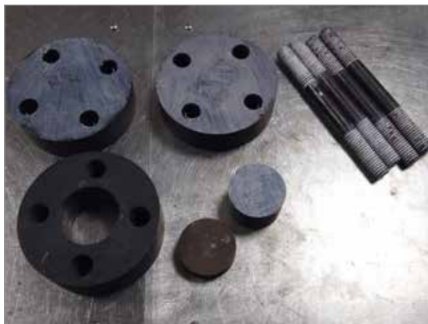
Figure 1 Round TEMTP A-286 plates, 718 cavity, dies and bolts
