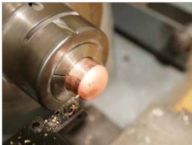
Figure 12 5C lathe being used to cut off the end of deep-drawn shape
