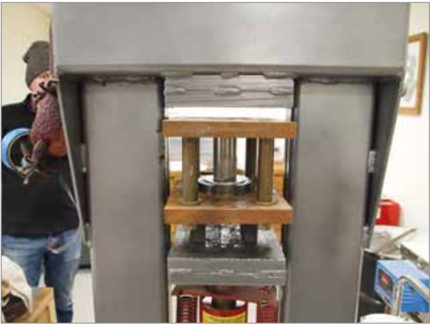
Figure 7 Die shoe used to align deep draw tooling in press
