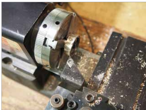
Figure 30 Dimensioning a patterned ring on a lathe
