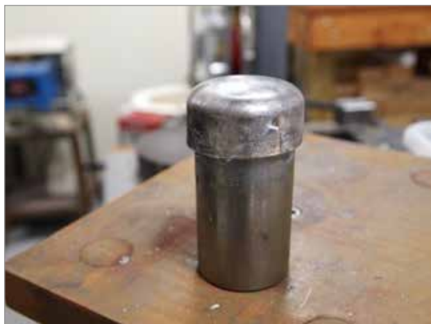
Figure 9 First draw of 3 mm plate forming cup shape
