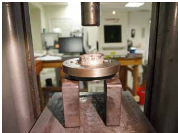
Figure 11 Second draw setup. Note top die being used as guide.
