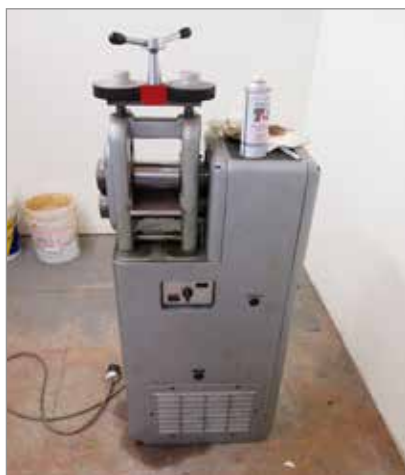
Figure 6 Rolling mill used for sheet reduction
