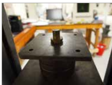
Figure 25 Ring-ironing die set mounted in press, inverted for tapered punch removal
